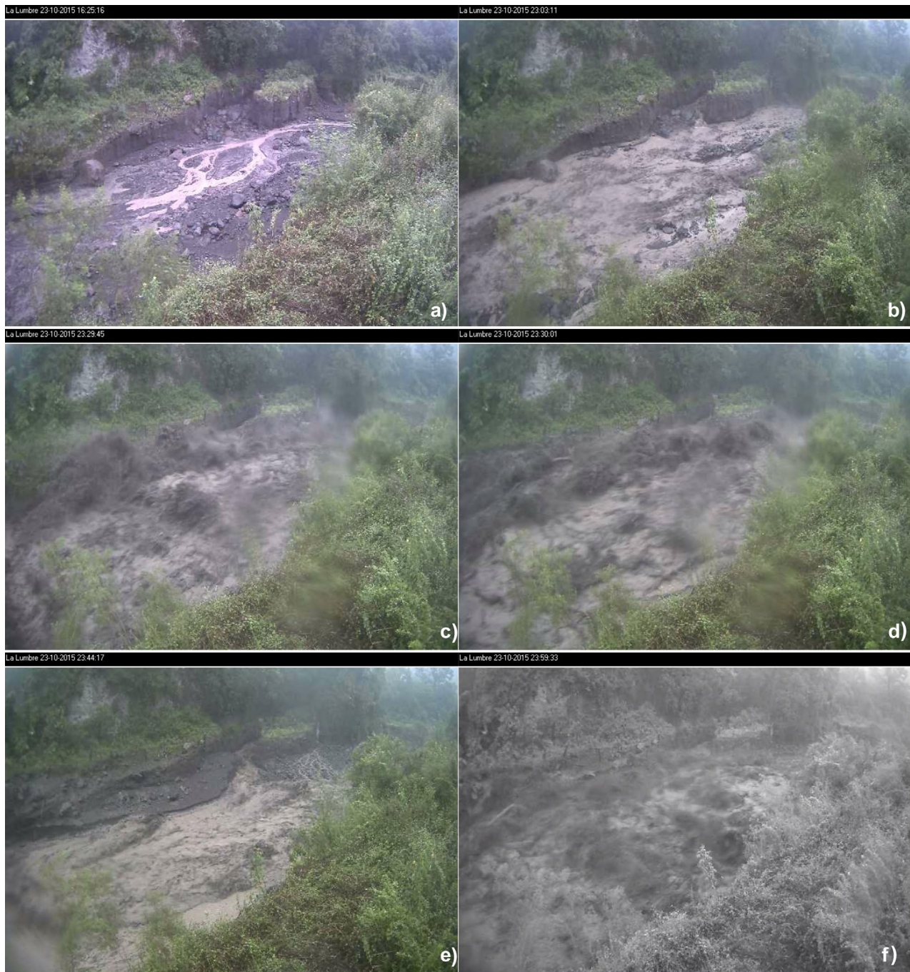
Figure 5. Selected frames acquired with the video camera at the Lumbre monitoring site. a) First stream flow; b) transition to hyperconcentrated flow; c and d) a1 front; e) hyperconcentrated flow between main fronts; f) a2 front.
