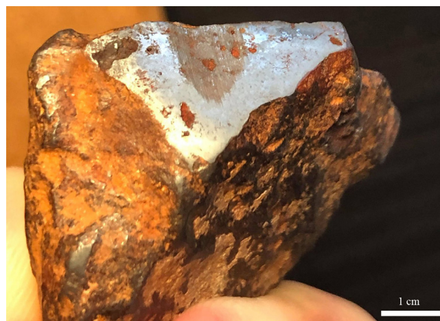
Figure 8. MNHNCu specimen from Cueva del Gato Jíbaro, Matanzas, western Cuba, believed to be meteoritic but resulted to be hematite aggregate. Scale = 1 cm.
