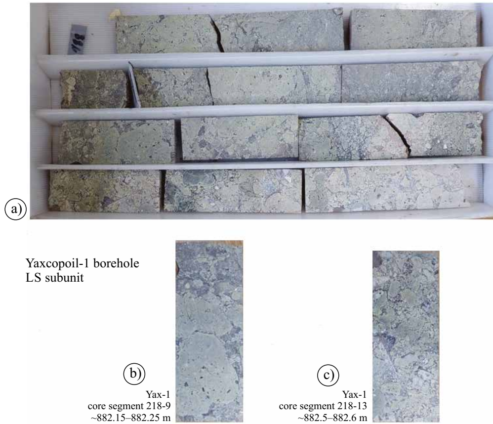
Figure 3. Images of Yaxcopoil-1 borehole core segments illustrating the textures, clasts and matrix in the Lower Suevite subunit. For scale, core diameter is 63.5 mm. (a) Yax-1 core box 218, (b) Yax-1 core segment 218-9, (c) Yax-1 core segment 218-13.
